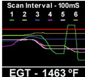
The temperature displayed is that of the hottest cylinder.
