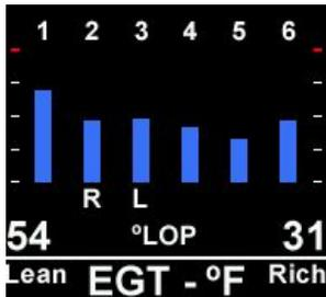
The cylinder with the “R” letter beneath it is the richest cylinder and the “L”, the leanest.
