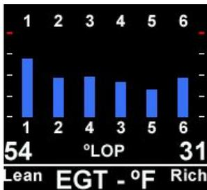
All cylinder conditions (LOP) will be between the values of the lean and rich temperatures. Your engine mixture has now been set to the desired LOP value.
