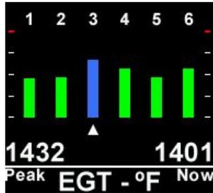
The first cylinder to peak will be displayed in blue with an arrow beneath it. **STOP LEANING.**
