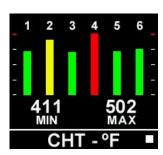
Displays the temperature of all cylinders in a graphic format. Colors are determined by the values set during installation.
