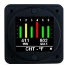
Six cylinder CHT systems and probe configurations
