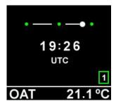
At the time of the interval period, the interval timer notification will be displayed on the bottom right in a green box. The value in the box is the minute value of the interval.
