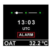
The instrument has a total of eight external alarm inputs. When an alarm condition is sensed the ALARM notification will be displayed on the current screen.
